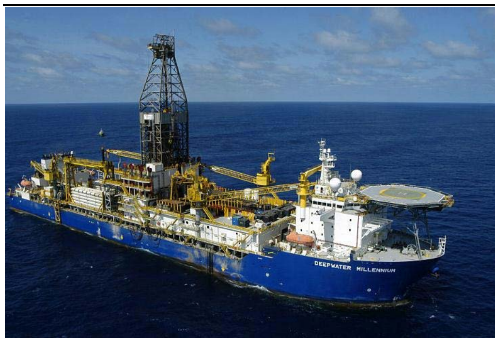
Figure 4.7 Example of a Dynamically Positioned Drill Ship
